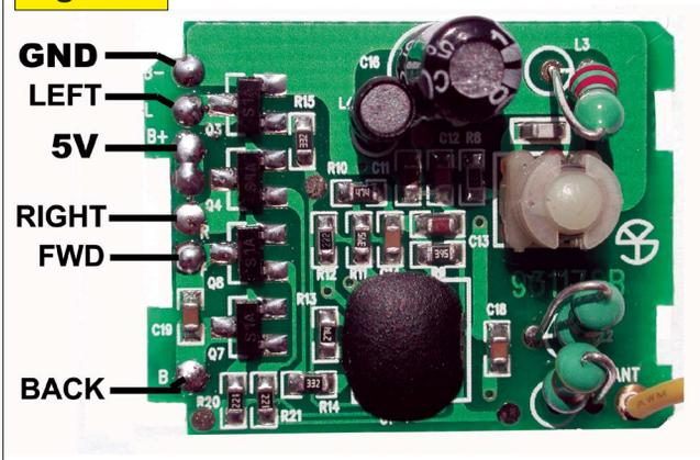
On opening up the car, I found a tiny receiver board operating from an equally tiny battery that was marked 1.2V 100 mA. My first concern was that I would want to get a useful signal level out of the device in order to interface to five-volt logic devices. I removed the battery
