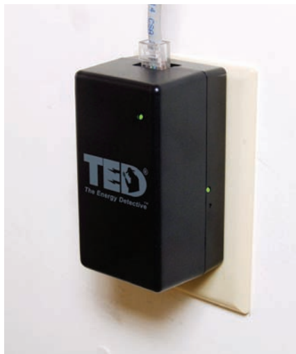
Left: TED Gateway is plugged into the wall, to receive data from its circuit monitors.
