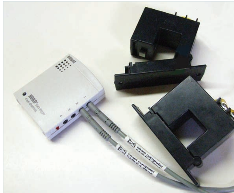
The HOB0 data logger with current sensors.
