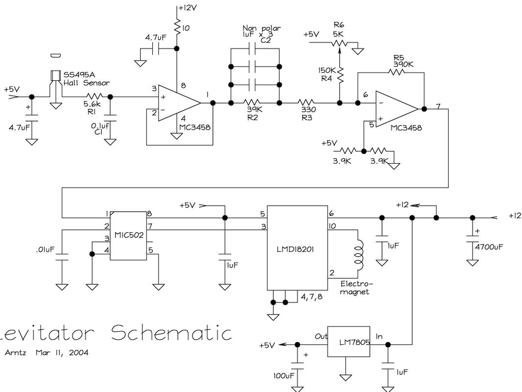
This way it remains cool, drawing maybe 0.25 amps or so DC, typically. It can sit there all day like that. The bridge IC has internal diodes for shorting out the otherwise destructive spikes from the electromagnet during the 1 kHz switchover.
